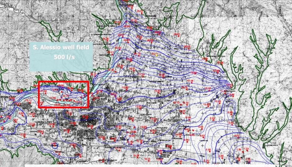
Along the Serchio River groundwater is pumped enhancing riverbank filtration into the sand and gravel aquifer. At Sant'Alessio, River head is artificially raised and 20 pumping wells withdraw about 600 l/s.
